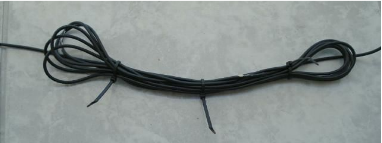
Image showing correct method to bundle excess cable length of the GPS Antenna
